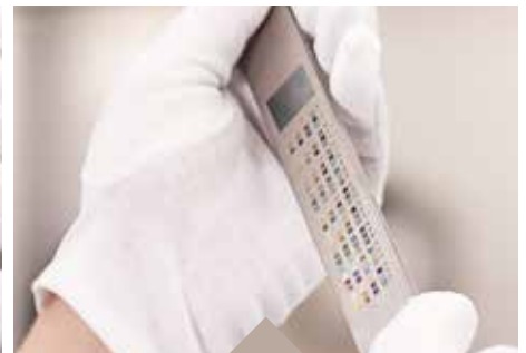
possible colour spectrum on titanium for laser engraving using the annealing method
